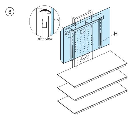
8-After mounting the brackets (H) to TV, hang TV onto holder (F), see (7-A).
